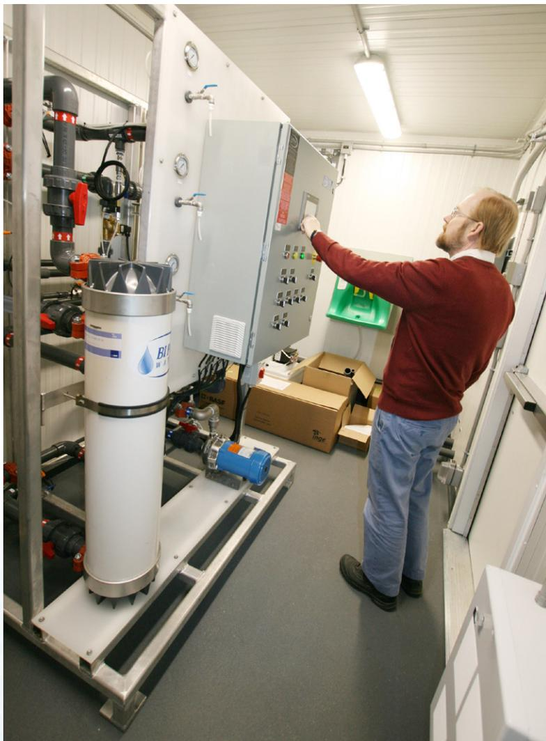
*A higher capacity UF package plant, with chlorine and air injection systems for the membrane backwash, is prepped for shipping*
