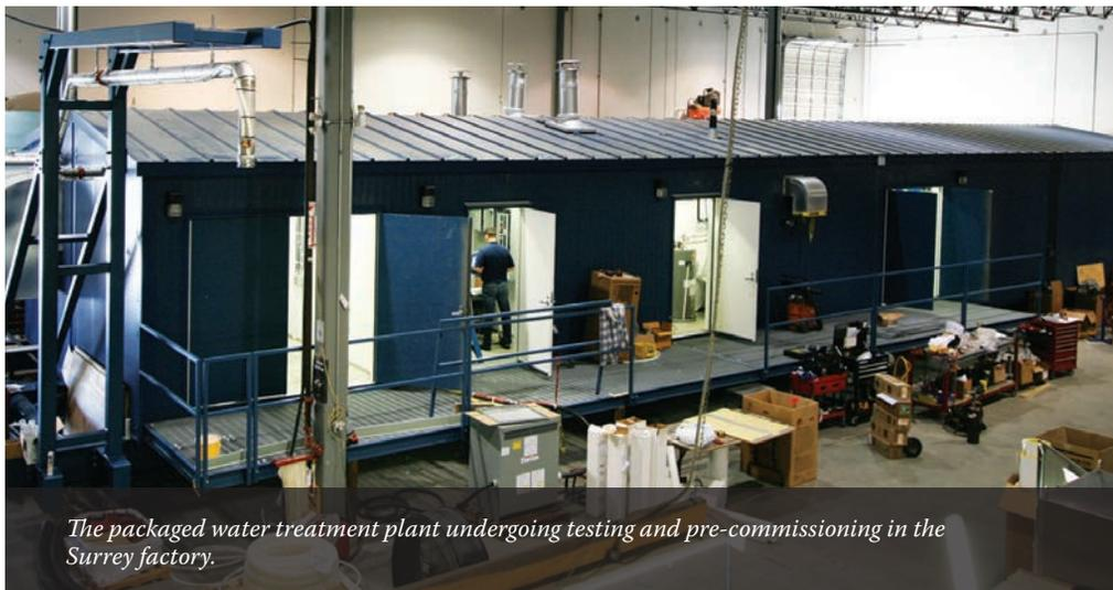
struction of modular units and pre-testing in the factory. This is followed by loading and shipping, site delivery, assembling on site, commissioning, operator training, and ongoing support.
