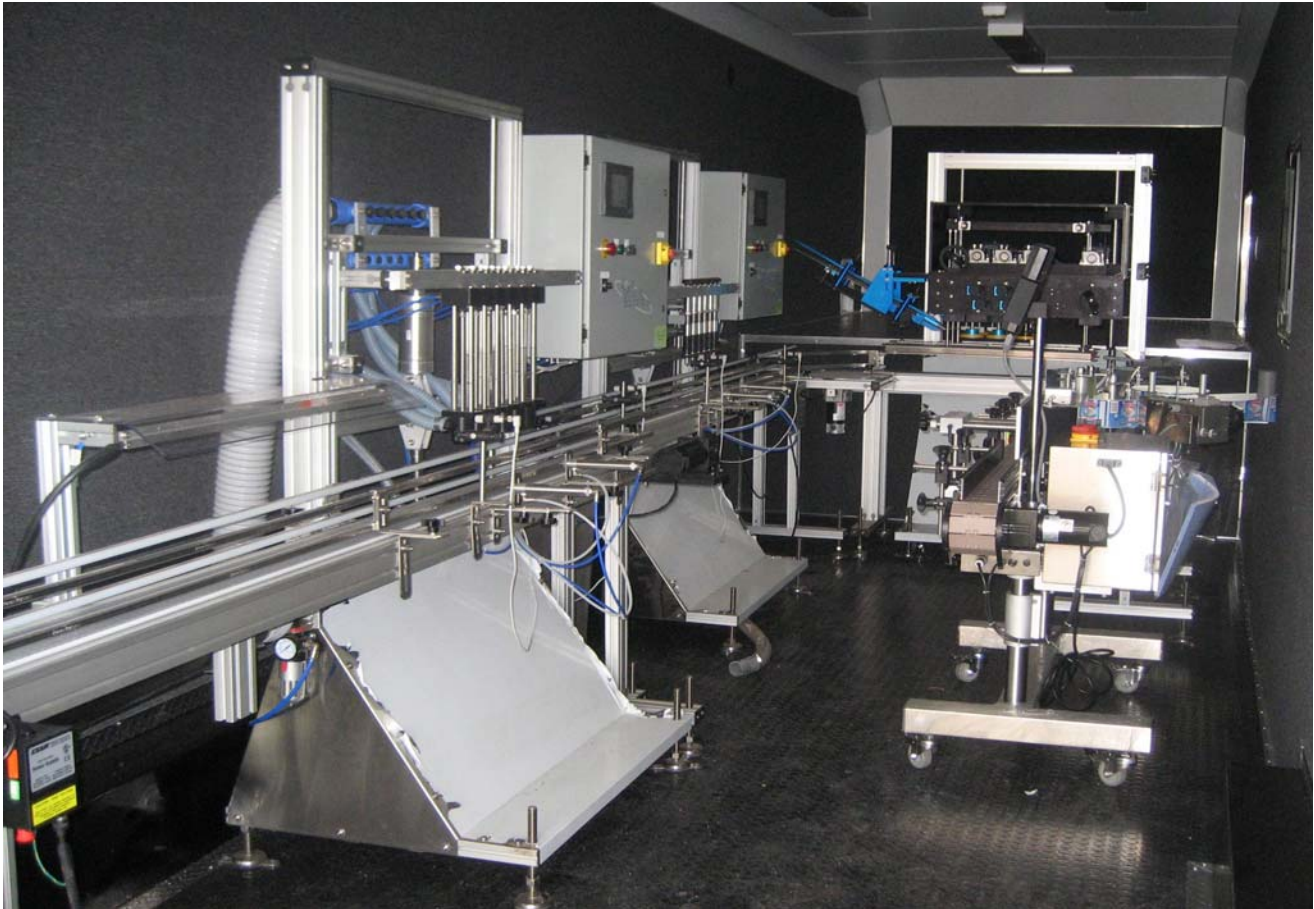
Figure 2 - From left to right is the bottle washer, filler, capper and labeler
